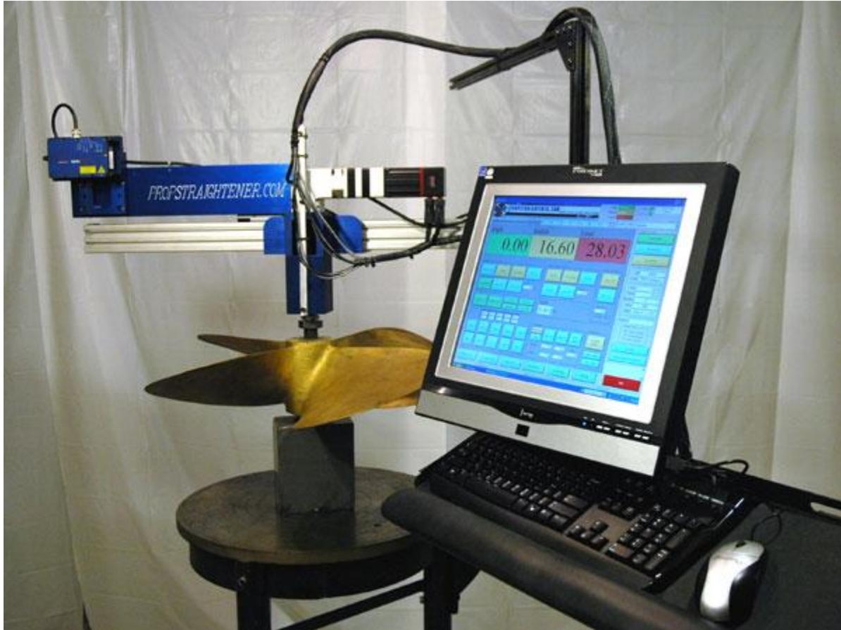
The system is designed to assess the repair status of propellers between 7.25" (184.15mm) and 63" (1600.2mm). The system does this by performing an automated scan of the propeller and calculating the pitch, rake, tracking and squareness of the propeller then comparing those results to ISO specification 484/2 to determine the classification of the propeller.
